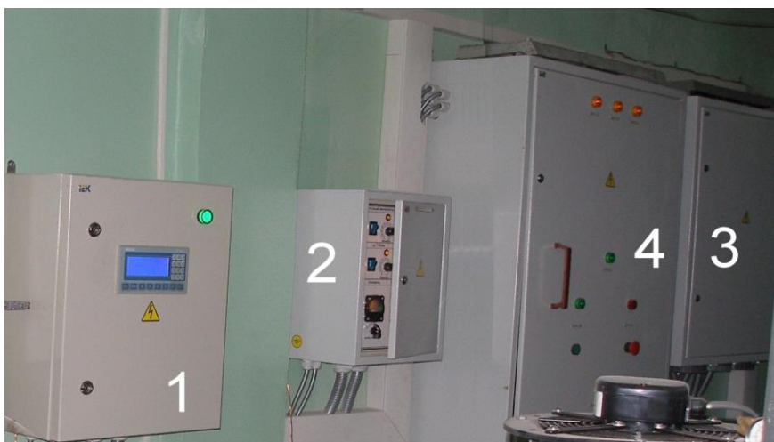
Fig. 1. Universal unit for drying and smoking products with automatic control system: 1 – automatic control unit; 2 – manual control unit; 3 – power unit; 4 – distribution unit (source: compiled by the authors)
